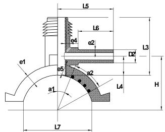
e4: minimum thickness of the saddle stack
